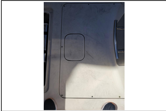
Gas Tank AFT Hatch SEALED
