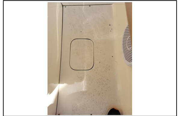
Gas Tank FWD Hatch SEALED
