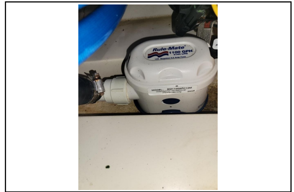
Bilge Pump FWDjpg
