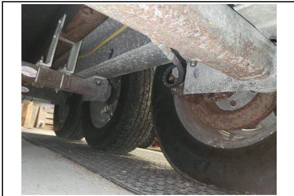
Trailer-corrosion to a minimum, tire thread good,
